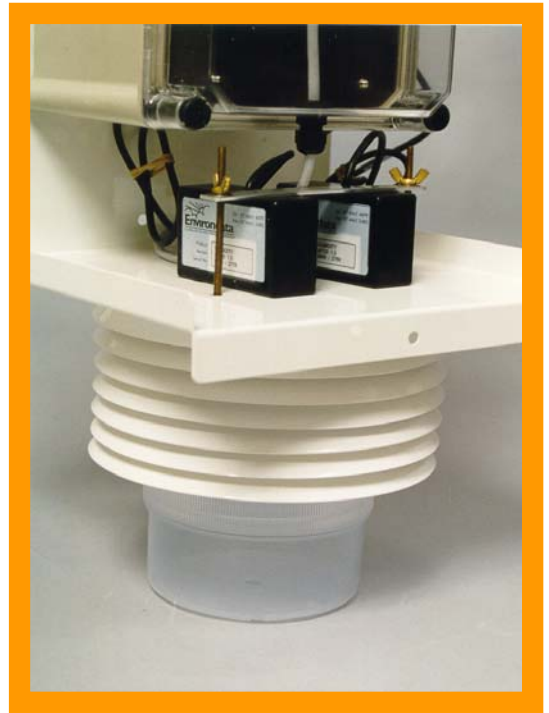
Two Temperature sensor as shown, One Wet & one Dry make up the Wet & Dry Humidity
