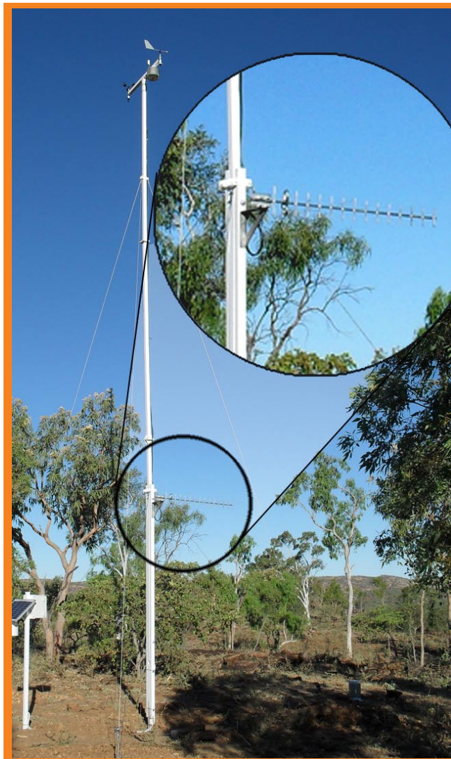
NG35 in a Weather Maestro System with directional high gain antenna
